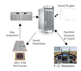
Fig. 1. Schematic of Neural Flight Control System using living rat cortical neurons for pitch and roll control.
